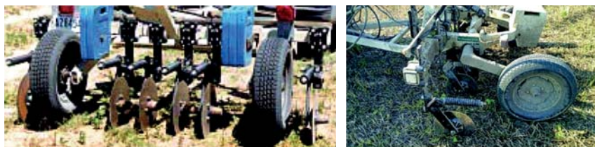
Slika 1. Skener elektrovodljivosti tla Veris EC Surveyor 3150 Figure 1. The scanner of soil conductivity Veris EC Surveyor 3150
