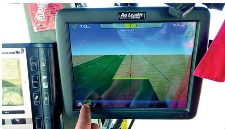
Slika 2. Prikaz prohoda traktora i rasipača na monitoru Integra Figure 2. The tractor and spreader on the monitor Integra
